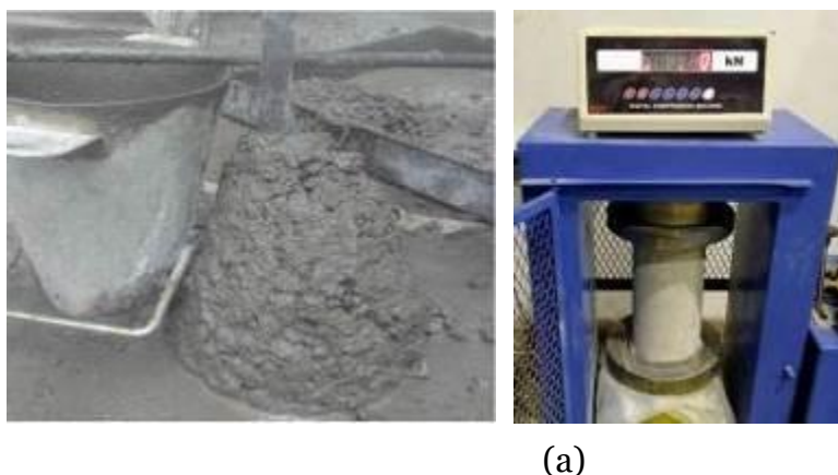
Fig 4. Testing programs on fresh and hardened concrete: (a) slump test to determine the workability of fresh concrete; (b) compressive strength test setup
