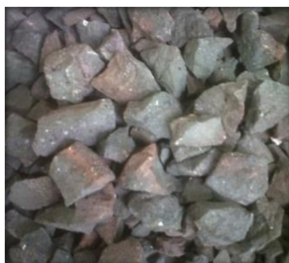
Fig 3. Crused clinker aggregate with a size of 2.36 mm to 19 mm
