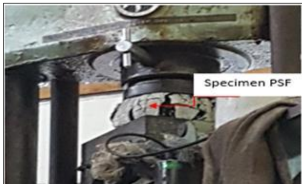
Fig 4. Specimen SFP after damage
