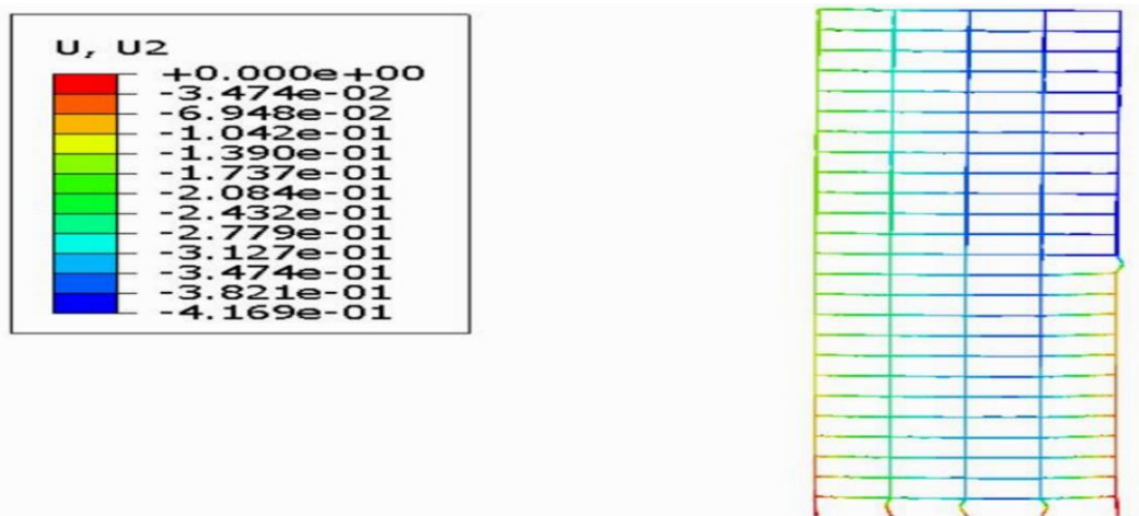
Figure 22: The highest displacement in thermal analysis in model number 20 (simple frame, 25-floor model, fire location next to the middle floor of the structure)
