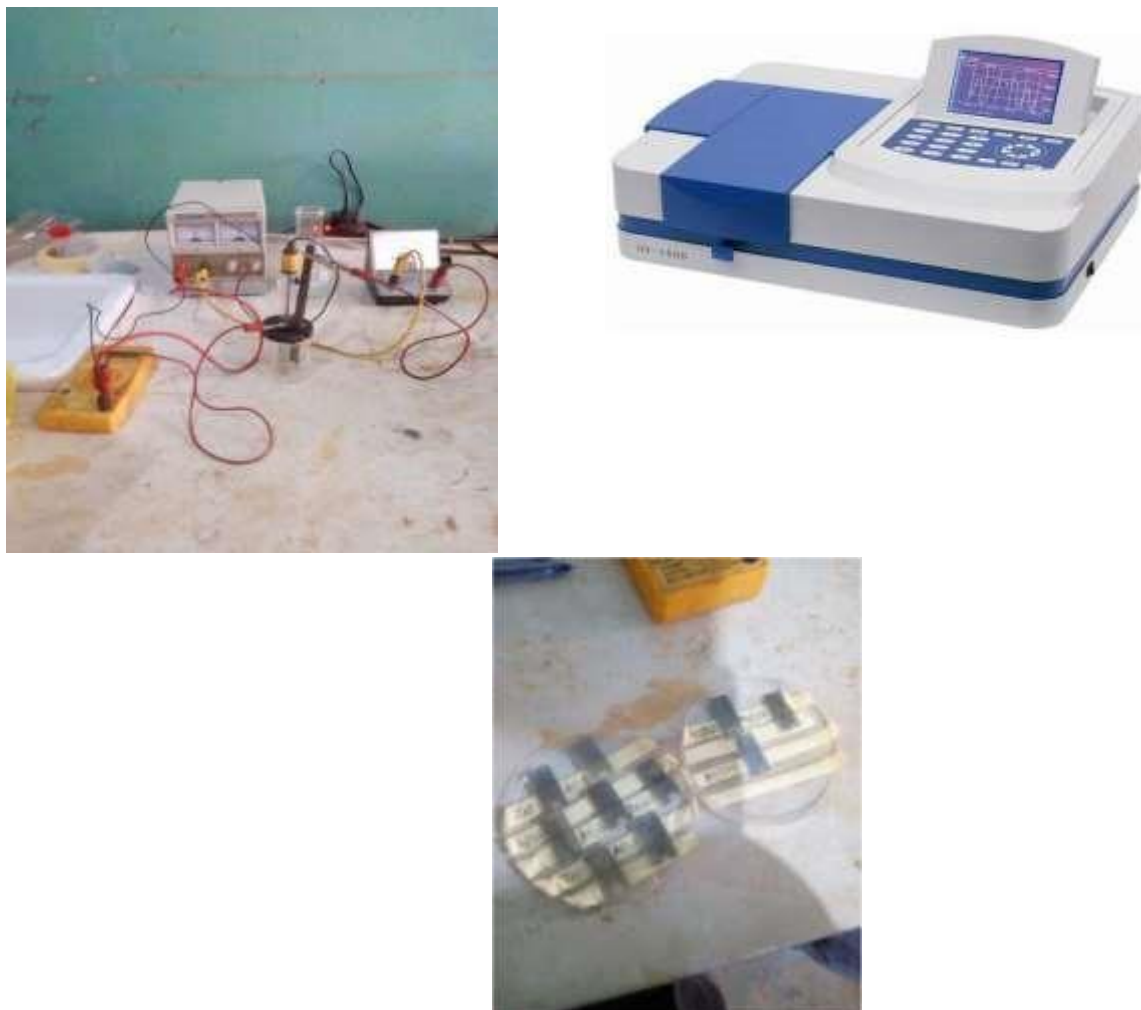
Figure 3.1 a) Electro deposition Machine b) UVs Spectrometer, C) Glass slides.
